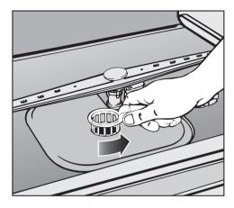
■ Turn the handle anti-clockwise to release the filter combination.
